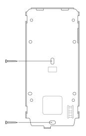
If installing BioStation 3 on a concrete wall, drill holes, insert PVC anchors, and fix them with fixing screws.
